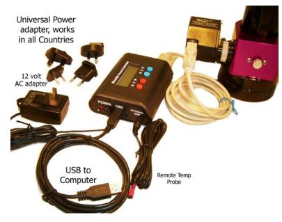
into the controller to bypass the built in temp probe located inside the case. Once plugged in, it will defeat the internal temp sensor. The probe can be taped to the side of the telescope for better thermal reading of the OTA.
