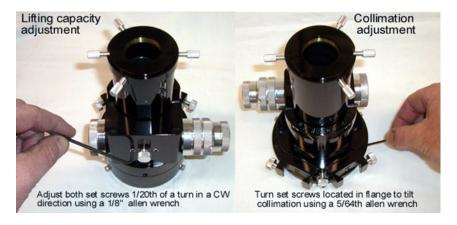
Lifting Capacity: The drawtube pressure can be adjusted to each user's preference. Increasing the pressure increases the load capacity (vertical lifting capacity) of the focuser. Decreasing the pressure lowers the load capacity but gives the focuser a smoother focusing action. We set the focuser at approximately 5 lbs. at time of assembly; however, you can adjust it to be more depending on your specific needs. The ideal setting is to have
