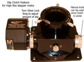
In most cases, the stepper motor option is picked at the time of focuser purchase; however, we do offer a user installed High Resolution Stepper Motor Kit for existing MoonLite focusers. The kit comes with different mounting brackets to fit different MoonLite focuser models. Please see our web site for additional kit information showing the different brackets available for different model MoonLite focusers.
