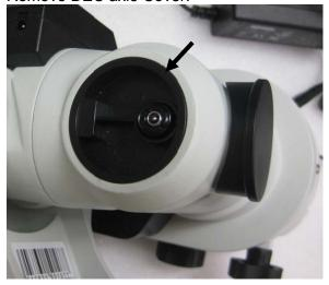
2. Unthread the illuminating LED with its plastic washer
