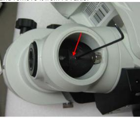
4. Point the polar scope to a far distant object. Adjust the Objective Lens by turning the tube to get a clear image. Tune the Lock Ring to secure it.
