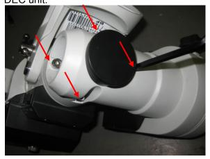
After fully releasing these screws, gently pull the DEC unit away from the RA axle to separate it from the mount. The polar scope will be fully exposed.
