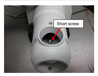
7. Put the DEC unit back onto the RA axle, with screw holes aligned to the threads on the RA axle. Gently thread the top screw into the threaded hole. It should feel very smooth without any difficulty. Then put two longer screws into the side holes and gently threaded
